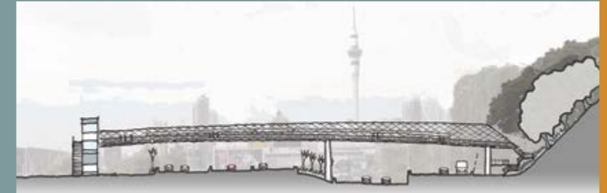
Three possible design approaches were identified in the initial draft Urban Design Framework for the pedestrian bridge including this Gantry Bridge Option. Source: Vic Park Tunnel Draft Urban Design Framework October 2006
