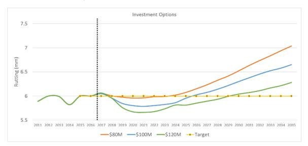
Rutting on the state highways is used as an indicator of pavement performance and expected life. As rutting deepens, other symptoms of deterioration are commonly present which signal that intervention treatments are required. Robust renewal and maintenance modelling has been undertaken on the state highway network. The modelled process has tested many different levels of investment to determine the optimum level, and the results have been verified.
