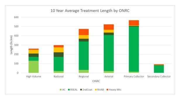
The investment model<sup>1</sup> selects the most economic treatment type over the long term. The high volume roads are predominantly constructed and treated with asphaltic concrete. Reseals are the most common treatment for other classes of road.
