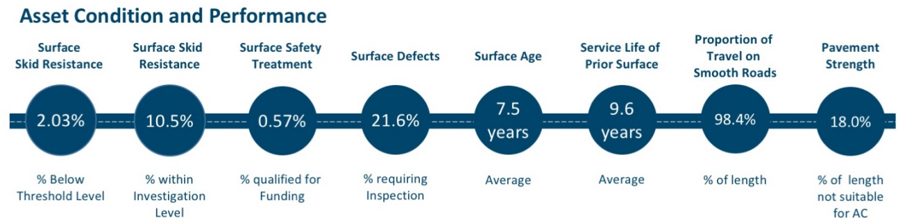
Figure 17 - Asset condition and performance
