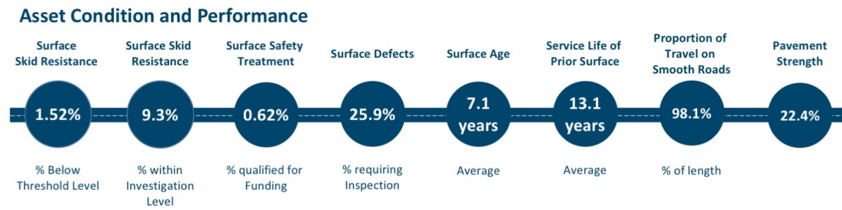
Figure 17 - Asset condition and performance
