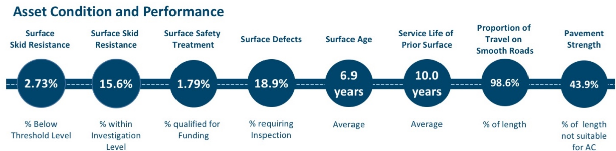
Figure 16 - Asset condition and performance
